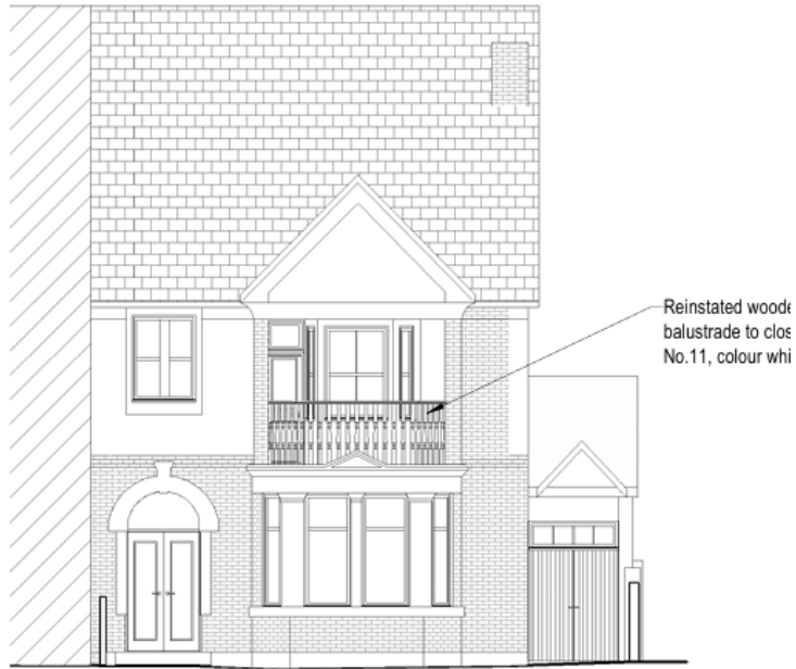
5 Proposed West Elevation 1 : 100
